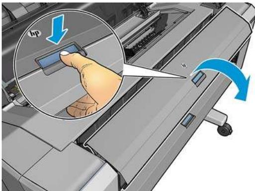
6. Manually rewind paper onto the roll.
