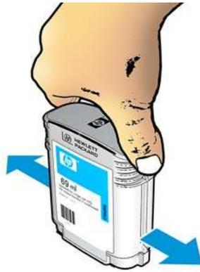
2. Unwrap the new ink cartridge, find the label identifying the ink color. Check that the letter or letters (in these illustrations, M for magenta) marking the empty slot, matches the letter or letters on the cartridge label.
