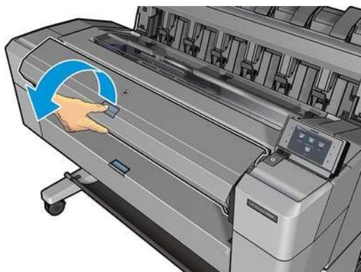
4. Load the spindle into the printer, with the blue stop on the right. Hold the spindle by its ends and not in the middle, to avoid touching the paper and perhaps leaving marks on it.
