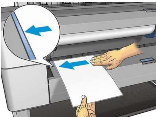
7. Push the sheet into the printer until it will not go any further.
