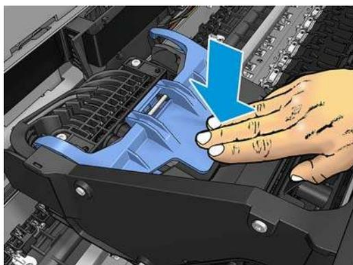
When the printhead has been inserted correctly and is accepted by the printer, the printer beeps.
