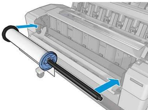
5. If the edge of the roll is not straight or torn (sometimes due to tape used to hold end of the roll), pull the paper slightly and cut a straight edge.
