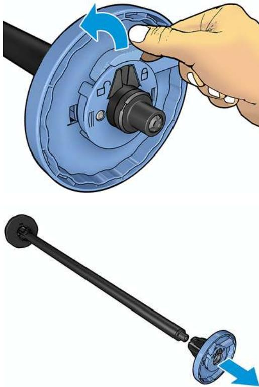
4. If there is already a roll or core on the spindle, remove it.
