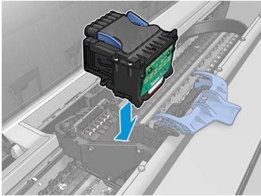
2. Check that the printhead is correctly aligned with its ink connectors.
