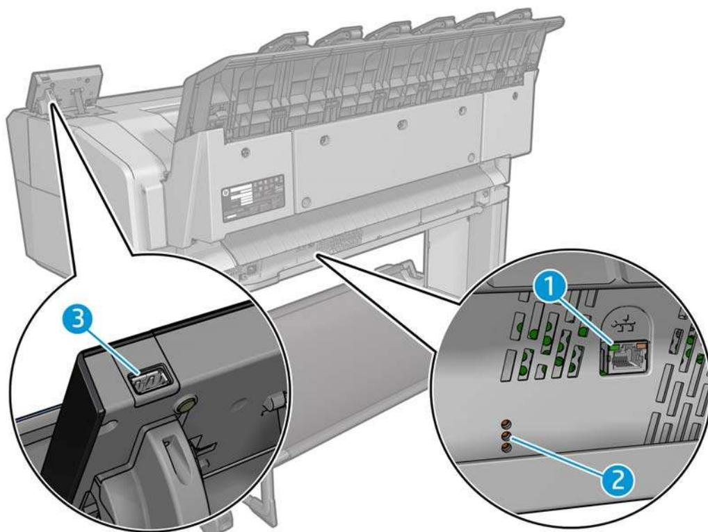
1. Gigabit Ethernet port, to connect to a network
