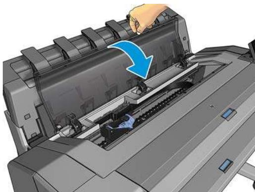
6. The front-panel display confirms that the printhead is correctly inserted. The printer starts checking and preparing the printhead. The default routine process takes 10 minutes. If the printer finds problems in preparing the printhead, it takes longer, up to 45 minutes. After the printhead is checked and prepared, the printhead realignment procedure runs automatically if paper is loaded, see [Align the printhead on page 177](#).
