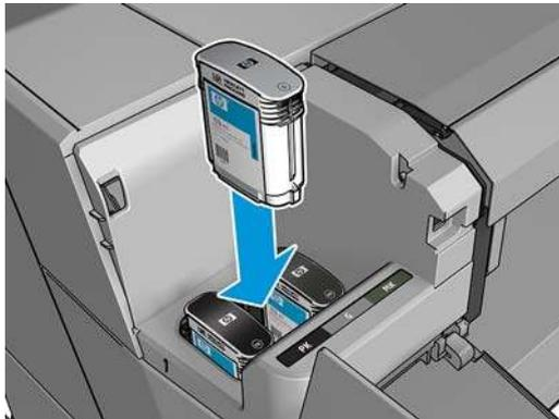
4. Push the cartridge into the slot until it snaps into position. You should hear a beep and see confirmation that the cartridge has been inserted.
