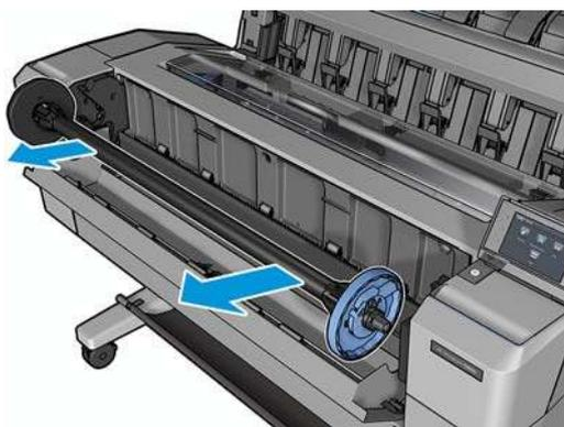
3. The spindle has a stop at each end. The blue stop can move along the spindle and has a latch to lock it in place. Open the latch and remove the blue stop from the end of the spindle.
