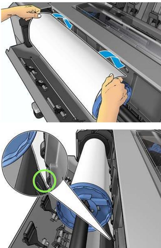
7. Roll the paper into the printer until you feel resistance and the paper flexes slightly. When the printer detects the paper, it feeds it in automatically.
