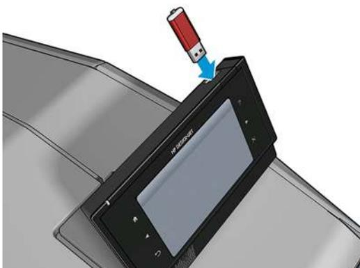
4. The printer takes about a minute to read the firmware file, then asks you to remove the USB flash drive.
