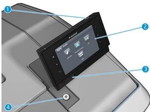
1. A Hi-Speed USB host port, intended for connecting a USB flash drive, which can provide files to be printed. When a USB flash drive is inserted, a USB icon
