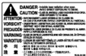
This machine has been classified under IEC 60825-1: 2007, EN60825-1: 2007 and conforms to the following classes:
