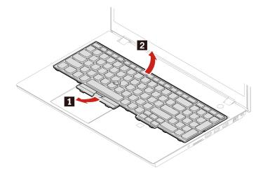
4. Put the keyboard on the palm rest as shown and detach the connectors. Then, remove the keyboard.
