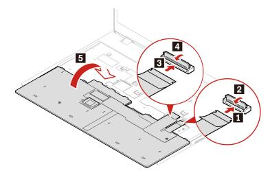
2. Insert the keyboard into the keyboard bezel as shown. Ensure that the top edge of the keyboard (the edge that is close to the display) is under the keyboard bezel.
