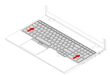
3. Pivot the keyboard slightly upward as shown by arrow **I** and then turn the keyboard **I** over.
